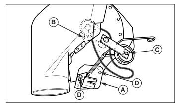
Figure 16. Belt Routing - 50" Models
